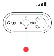
Bottom LED is RED. Select speed and good to go. Then just volume to adjust sound level
